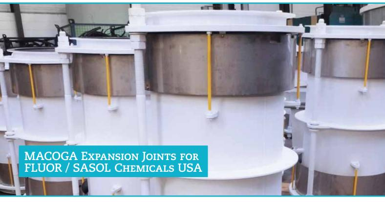
MACOGA has designed, manufactured, tested and delivered one Lateral tied DN2600, 12 DN800 and one **Rectangular** MRU 2000 x 630 expansion joints to Fluor for Sasol Chemicals in the USA.
