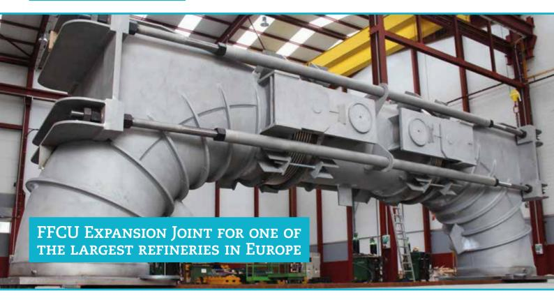
MACOGA has successfully designed, manufactured, tested and shipped a large tied universal FFCU expansion joint for one of the largest crude oil processing locations in the North of Europe.
