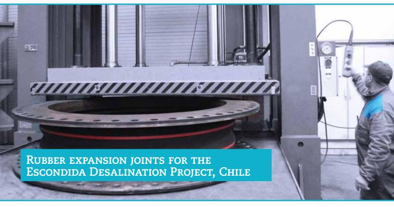
MACOGA has designed, manufactured, tested and delivered a large number of MAC-F2 DN1500 expansion joints for the Escondida Water Supply Project in Chile. Each expansion joint incorporates a Double Arch EPDM bellows and Superduplex S32750 flanges.
